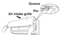
Press in the bottom right and left corners of the air intake grille to attach the indoor unit.
